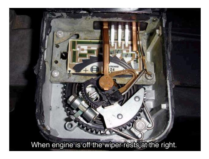
When the engine is running the wiper moves to the left (idle position) and this allow the fuel pump contact on the right to close:
