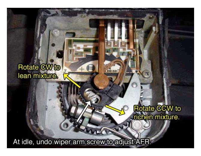
Adjustment is simply a matter is undoing the wiper screw and rotating the wiper slightly. The only hard part is keeping the wiper from moving while you retighten the screw. This is less of a problem if you can't detect small changes in the mixture. When you are done, drop some silicone or a drop of purple loctite where the screw meets the slot underneath.
